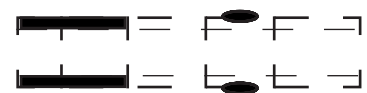
Diagram C (cut away blacked out section and snip in at scored sections up to the 1/4” mark. use an oval punch as indicated.)
